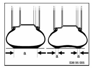
Figure 5: Cross-section of a tyre with too high and too low an inflation pressure
