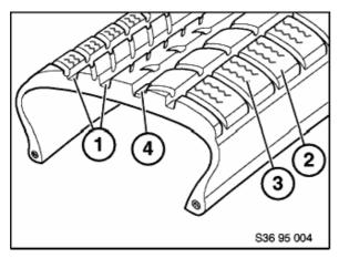
Figure 4: Illustration of tyre tread with lugs, grooves and slits
