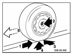
Figure 2: Forces acting on the wheel
