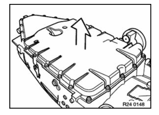
Unscrew bolts and remove oil pan.
