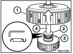
Remove B clutch (1), angled disc (2) and axial needle bearing (3) from idler shaft (4).
