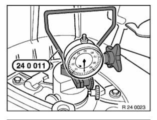
Fit and secure special tool 24 0 011 with dial gauge to the input shaft.
