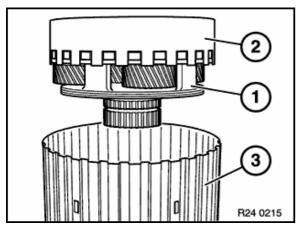
Remove planet spider I (1) and ring gear II (2) from ring gear I (3).
