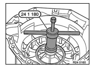
Clamp special tool 24 1 180 on stator shaft. Remove oil supply line from transmission case.
