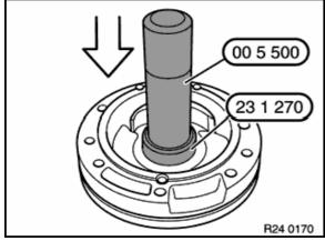
Press out seal and needle bearing with special tool 00 5 500 and 23 1 270 on hydraulic press.
