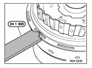
Do not reuse bent retaining tabs for securing purposes. Using special tool 24 1 300, first bend two opposing
