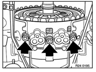
Screw special tool 24 1 260 into planetary gear set, tighten down knurled screw.
