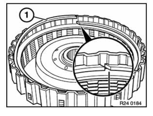
Lift out snap ring (1) from B clutch and remove complete disc pack.
