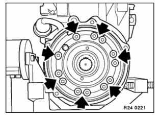
Arrange transmission horizontally. Unscrew bolts.
