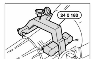
Secure transmission to assembly frame with special tool 24 0 180.
