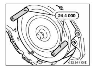
Screw special tool 24 4 000 into torque converter and remove torque converter.
