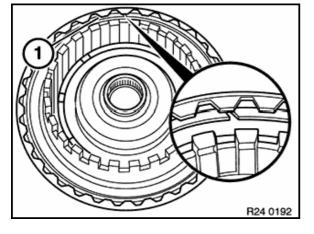
Lift snap ring (1) out of C clutch and remove complete disc pack.
