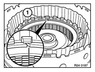
Lift snap ring (1) out of A clutch.
