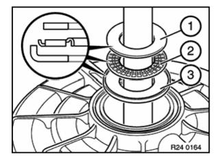
Remove adjusting disc (1), needle bearing (2) and angle disc (3).
