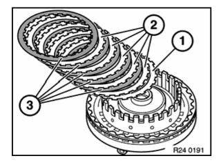
Remove complete disc pack from A clutch.
