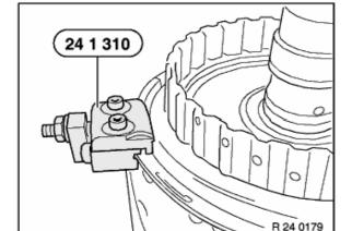
Bend back retaining tabs with special tool 24 1 310.
