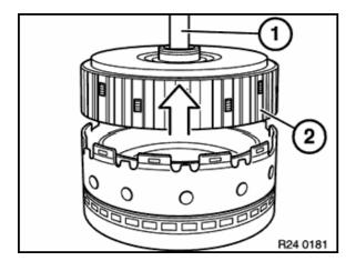
Lift off idler shaft (1) with clutch B (2).
