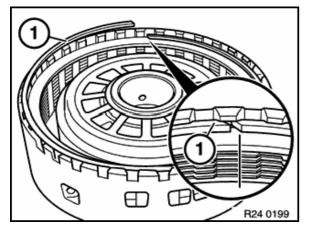
For ease of assembly, coat perimeter of cylinder D/E (1) with Vaseline
