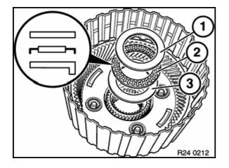
Remove thrust washer (1), axial needle bearing (2) and angled disc (3).
