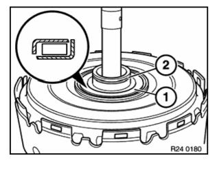
Remove axial needle bearing (1).
