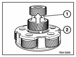
Remove sun gear II + III (1) from planet carrier III (2).
