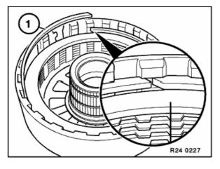
Lift snap ring (1) out of multi-disc brake F (2) and remove complete disc pack.
