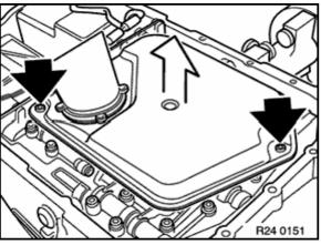
Unfasten screws and remove oil strainer.
