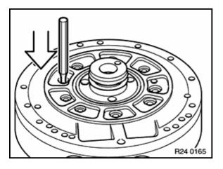
Remove oil pump from oil supply housing with cotter pin extractor and plastic hammer.
