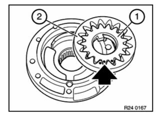
Remove pump wheel (1) and ring gear (2) from pump housing.
