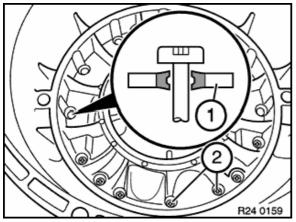
Unfasten all screws with large heads (12 off) Lift off shift unit.
