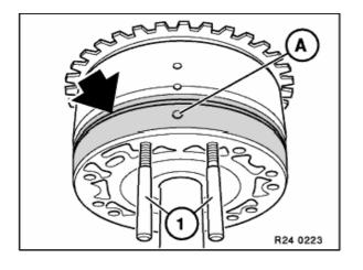
Screw the guide bolts (1) (2 bolts M8x70 without bolt heads) into cylinder F, each next to the bore (A).
