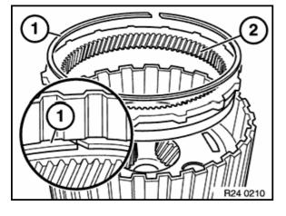
Place planetary gear set I + II on two wooden blocks Lift out snap ring (1) and remove ring gear III (2).
