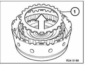
Remove end disc (1) from A clutch.
