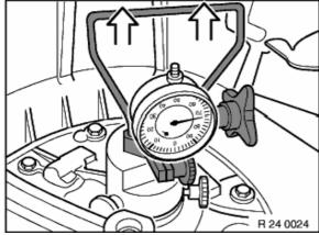
Withdraw input shaft as far as stop and read off measuring value.
