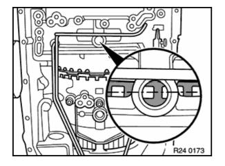
The impulse spring on the top clutch housing must be located in centre of bore for impulse sensor.
