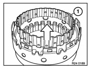
Remove internal disc carrier B (1).
