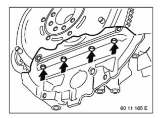
Release oil sump screws pointing to end cover and then remaining oil sump screws.
