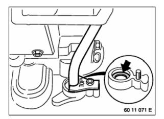
Remove guide tube for oil dipstick.
