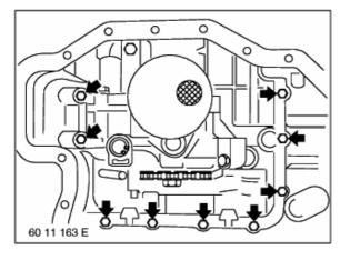
Release oil sump screws on inside of oil sump.
