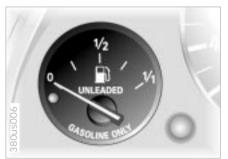
Please refuel early, since driving to the last drop of fuel can result in damage to the engine and/or catalytic converter.
