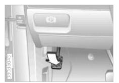
If, in exceptional circumstances, it should be necessary to engage the parking brake while the vehicle is in motion, depress the pedal cautiously and slowly while continuing to pull on the release handle.
