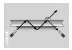
The rain sensor controls windshield wiper operation, depending on how wet the windshield is.
