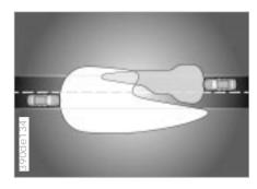
The xenon lamps light up the side and front areas of the vehicle with significantly more brightness and uniformity than the traditional halogen lamp.
