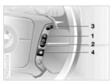
You can store and automatically maintain any desired vehicle speed above approx. 20 mph (30 km/h).
