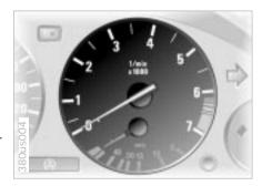
Never allow the engine to operate with the needle in the red overspeed zone of the gauge.
