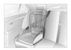
To allow you to use the safety belts to secure child-restraint systems, the belts at all rear positions feature a special locking mode.
