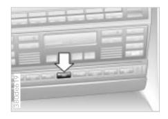
The PDC assists you when you are parking. Acoustic signals warn you of the distance to an obstacle. In addition, four ultrasonic sensors in each the front and rear bumpers measure the distance from the nearest object. The monitoring range for the four front sensors and that of the two rear corner sensors ends approx. 2 ft (60 cm) beyond the respective bumper. The two center sensors cover a distance of approx. 5 ft (1.50 m).
