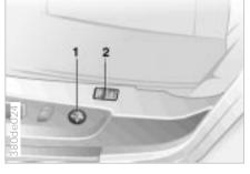
With this seat, you can also adjust the thigh support. Press the switch to make the adjustment.
