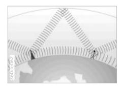
Radio waves – mediumwave, longwave and shortwave – offer a wide range of reception, because the broadcast signals travel not only along the ground as surface waves, but also as waves bounced back to earth from the ionosphere.
