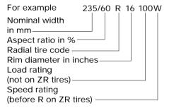
The speed rating indicates the approved maximum speed for the tire.
