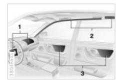
1 Front airbags for driver and front passenger
