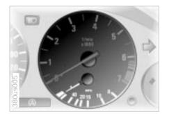
Indicates current fuel consumption in mpg (in liters per 100 km on Canadian vehicles). This instrument clearly shows whether your current driving style is conducive to economy and minimum exhaust emissions.
