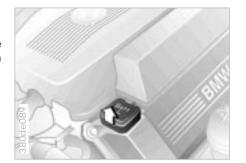
4 Start by connecting the jumper cable from the positive terminal of the support vehicle to the positive terminal connector located in your BMW's engine compartment. The cover of the auxiliary terminal for jump starting is marked with "Batt. +" (refer to the illustration). Open the cover by pulling the tab. The illustration shows the auxiliary terminal for jump starting the BMW 740i/L as an example. For the BMW 750iL: Refer to "Engine compartment" on page 146
