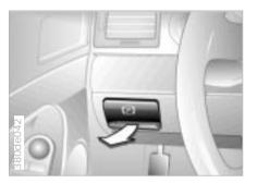
To release the brake, pull the handle. Please remember that the brakes disengage immediately.
