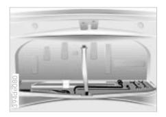
The onboard tool kit is located in the luggage compartment lid. Loosen the wingnut to open.
