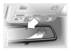
The semisolid reacts chemically to this electrical current, thus providing infinitely-variable dimming of the mirror (electrochromic technology).
