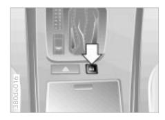
Use this button to operate the central locking system when the front doors are closed. With this button, only the doors and luggage compartment lid are unlocked or locked. The antitheft system is not activated.
