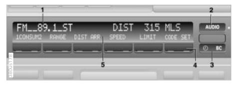
The onboard computer operates at ignition key positions 1 and 2.
