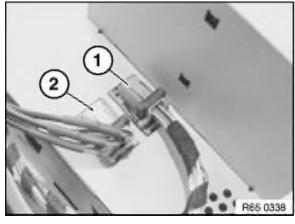
Unlock plug connections (1) and (2) and disconnect. Remove complete on-board monitor.
