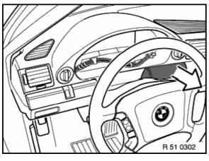
Remove top left wooden finisher by pulling upwards.
