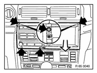
Unfasten screws and pull on-board monitor forwards to remove.
