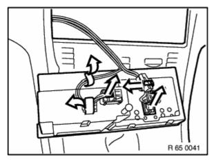
Remove plug and unfasten wiring harness from clips.
