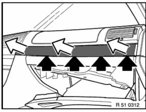
Release upper plastic nuts and remove wooden finisher.
