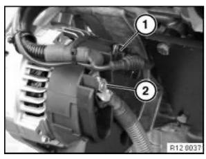
Connections illustrated here on removed alternator.
