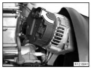
Pull alternator upwards to remove.
