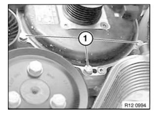
Release screws (1) on alternator.
