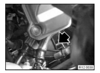
Disconnect alternator connections.
