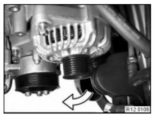
Unclip cooling air guide.
