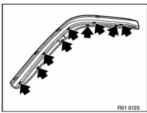
Unclip and remove chrome finisher from body molding.
