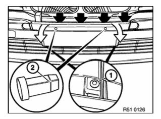
Lift out expanding rivets (1) underneath and expanding tapers (2) on top.
