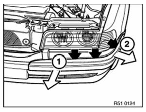
Unclip body molding with hardwood wedge and remove, first from front (1), then from side (2).
