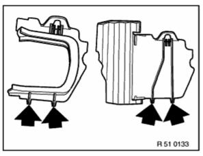
Unfasten top fasteners (1) and lift fresh air grill upwards and forwards to remove.
