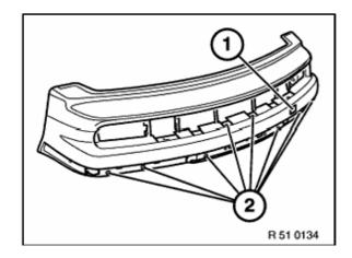
Lift cover (1) off towing eye and unfasten catch band. Lift out expanding rivets (2) and lift bumper carrier backwards to remove.
