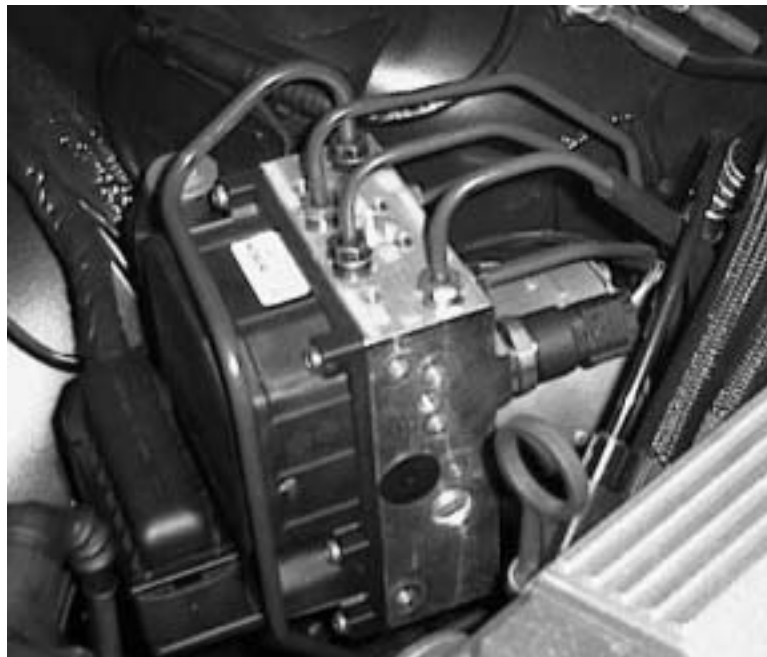
Control Module/Hydraulic Unit Bosch DSC III 5.7
