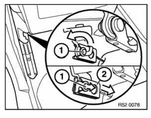
Pull retainer (1) backwards to unlock and pull inwards to remove. Lift Bowden cable (2) for seatbelt height adjustment forwards to remove.
