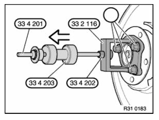
Pull off bearing unit with special tool 33 2 116 / 33 4 201 /202 / 203 and wheel studs (1).
