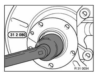
Unfasten nut with special tool 31 2 080. Do not reuse nut!
