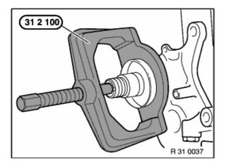
Inner bearing race can also be removed with special tool 31 2 100.
