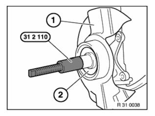
Fit guard plate (1). Fit new dust cover (2). Bore in dust cover must be aligned with bore in steering knuckle. Tighten special tool 31 2 110 firmly down.
