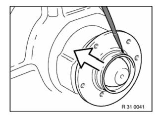
Install new cap with sealing compound, refer to BMW Parts Service.
