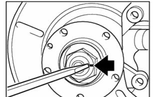
Peen down retainer on collar nut.
