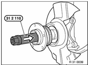
Slide on new bearing unit and fit using special tool 31 2 110.
