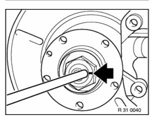
Tighten new collar nut to specified torque, refer to Technical Data 31 21 1AZ, and calk.
