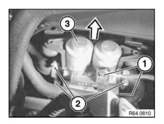
Unlock plug connections (1) and disconnect.
