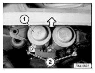
Pull water valve (1) in direction of arrow out of rubber mounts. Release hose clamps (2) and detach water hoses. Pull out water valve (1) in direction of arrow.
