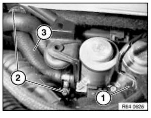
Unlock plug connection (1) and disconnect. Release hose clamps (2) and detach water hose (3) completely.
