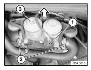
Unlock plug connection (1) and disconnect.
