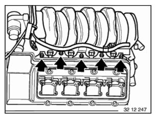
Unfasten nuts (left and right). Remove decoupling elements and lift intake air manifold upwards to remove.
