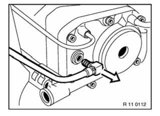
Remove connector for brake force booster.
