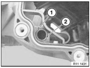
If necessary, remove vent pipe in intake air manifold: Remove throttle valve.
