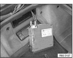
Disconnect plug connections and remove navigation computer.
