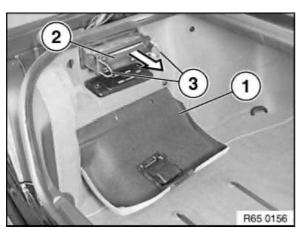
Open flap (1) in side panel, rear left. Release navigation computer (2) with special tool 65 5 400 (3) and pull out.
