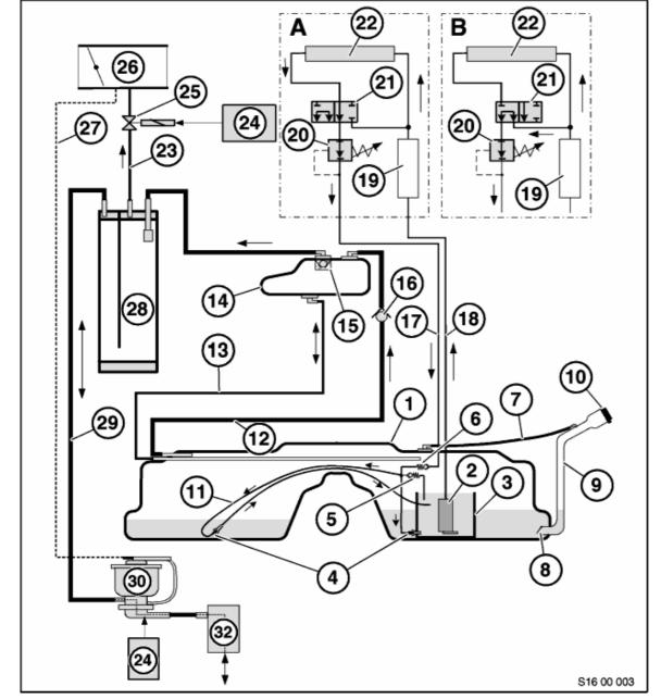
5.3 Fuel supply system E38 / E39 with M52 / M73 USA
