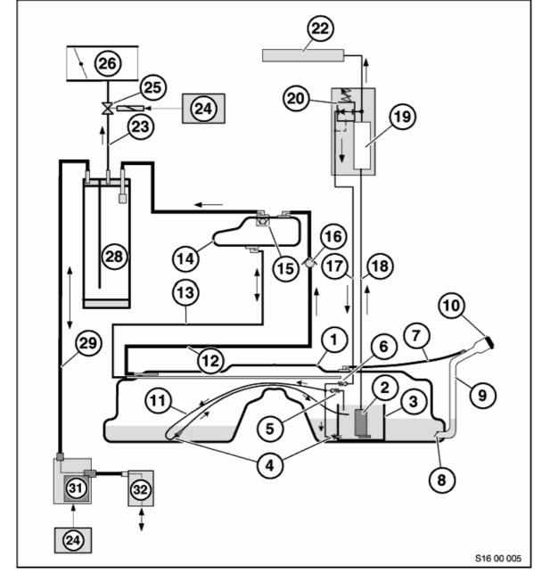
5.5 Fuel supply system E39 with M54 / M62 USA (DM-TL)
