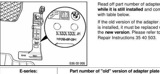
Read off part number of adapter plate while it is still installed and compare with table below.
