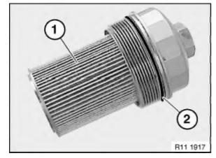
Detach oil filter element (1) from main flow oil filter cover and replace.
