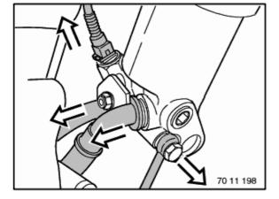
Disconnect plug connection on oil pressure switch.
