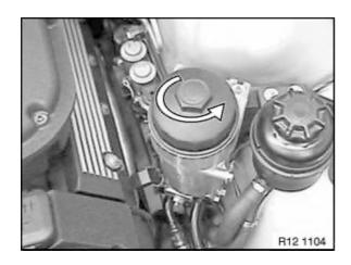
Open or tighten down main flow oil filter cap with a wrench socket.
