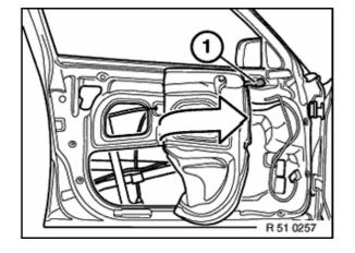
Detach sound insulation at rear until screws at bottom are accessible and secure with adhesive tape (1).
