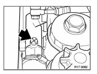
On vehicles with M52 engines, also unfasten additional vent screw.
