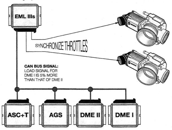
The EML control module processes the load signals from the two DME control modules. If a difference exists, the EML will adjust the DK motors to achieve equal air throughput on both banks.
