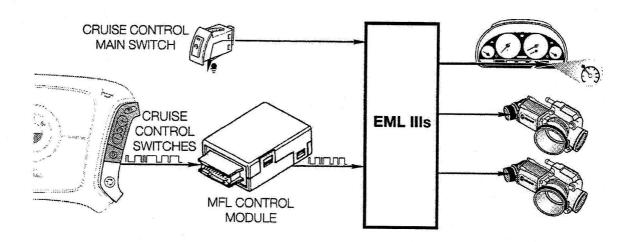
The EML controls the cruise control indicator lamp in the instrument cluster. When the main switch is pressed, the indicator lamp is illuminated.
