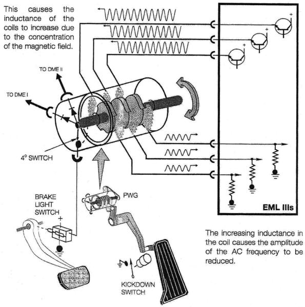
The amplitude is decreased linearly as the pedal is pressed down.
