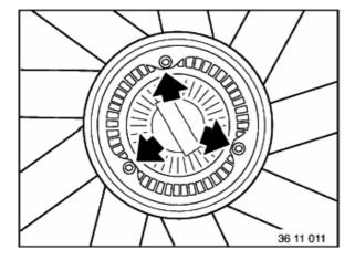
Unfasten screws and detach fan from fan coupling.
