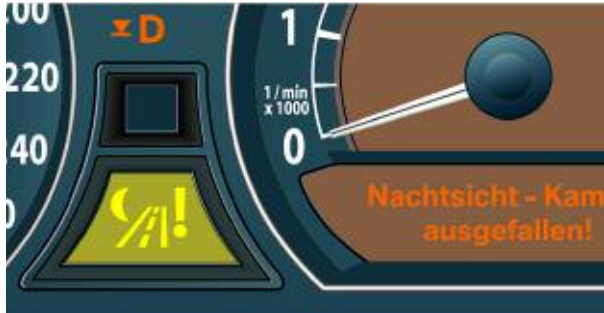
Displays in Event of a Fault (E65/E66)
