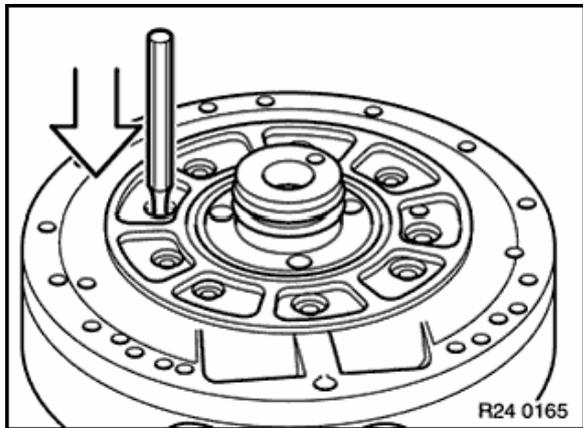
Remove oil pump from oil supply housing with cotter pin extractor and plastic hammer.
