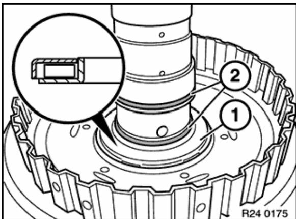
Place drive unit with clutches (A/B/C) on its head.
