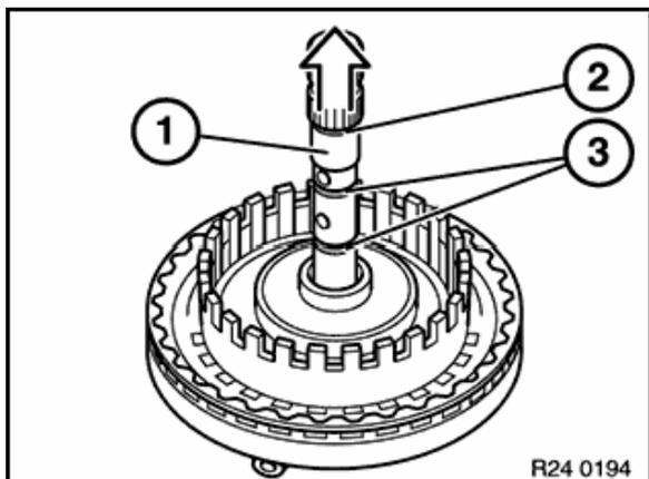
Press input shaft (1) out of cylinder A + C.
