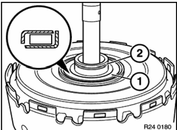
Remove axial needle bearing (1).
