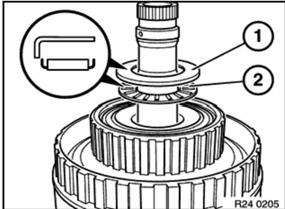
Remove angled disc (1) and axial needle bearing (2).
