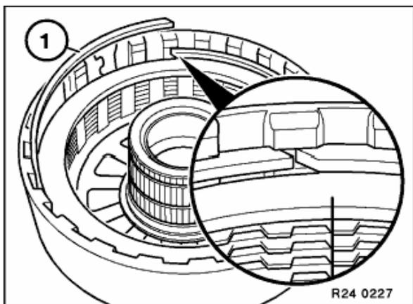
Lift snap ring (1) out of multi-disc brake F (2) and remove complete disc pack.
