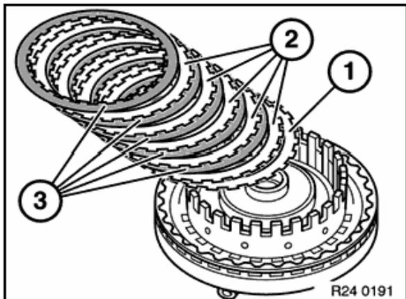
Remove complete disc pack from A clutch.
