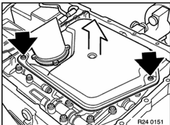
Unfasten screws and remove oil strainer.
