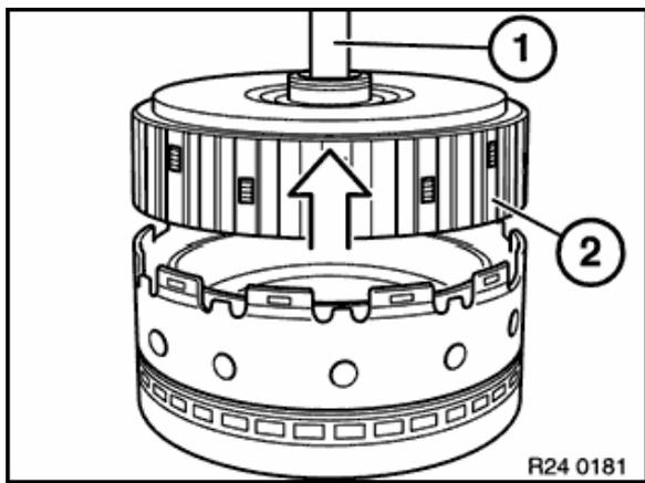
Lift off idler shaft (1) with clutch B (2).
