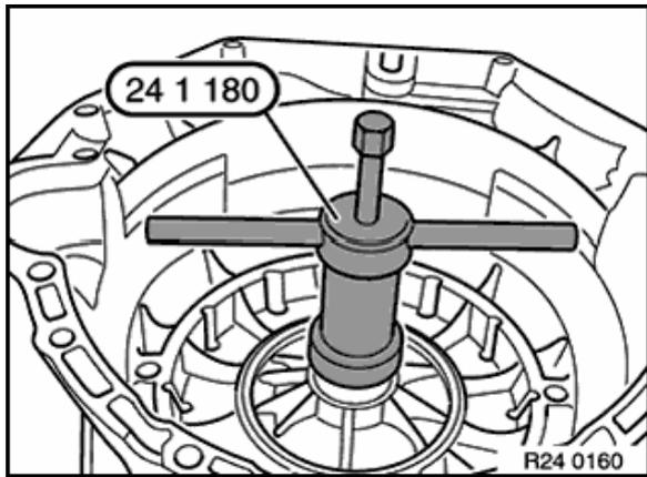
Clamp special tool 24 1 180 on stator shaft.
