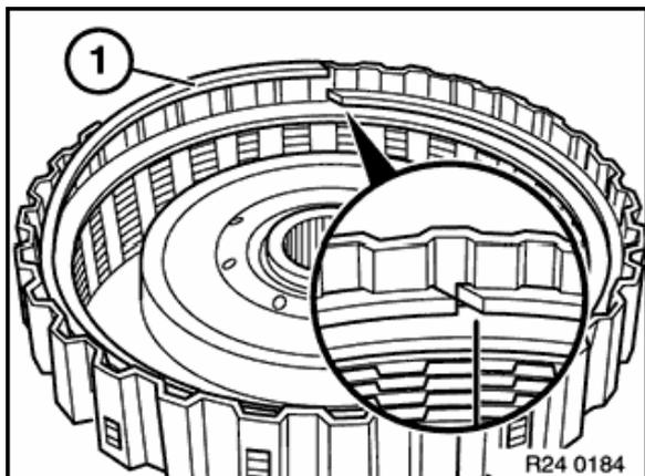
Lift out snap ring (1) from B clutch and remove complete disc pack.
