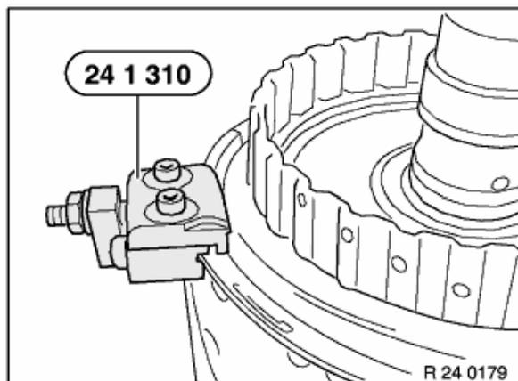
Bend back retaining tabs with special tool 24 1 310.
