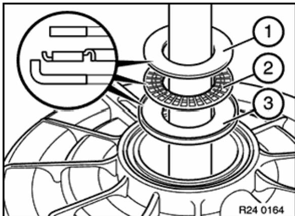
Remove adjusting disc (1), needle bearing (2) and angle disc (3).
