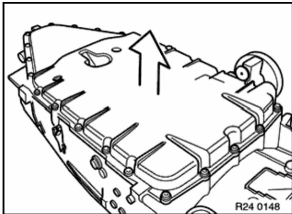
Unscrew bolts and remove oil pan.
