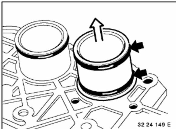
Remove suction and pressure pipes from shift unit and replace all O-rings.
