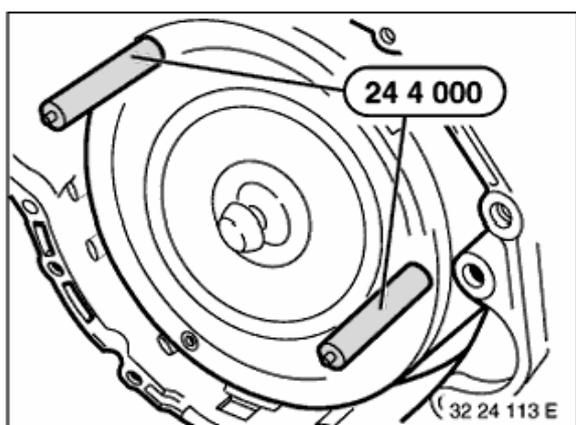
Screw special tool 24 4 000 into torque converter and remove
