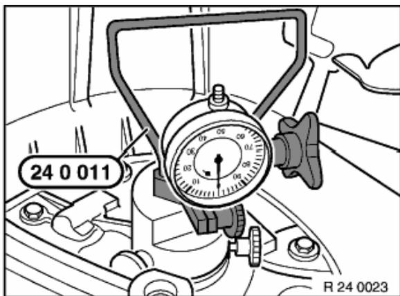
Fit and secure special tool 24 0 011 with dial gauge to the input shaft.
