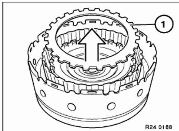
Remove end disc (1) from A clutch.
