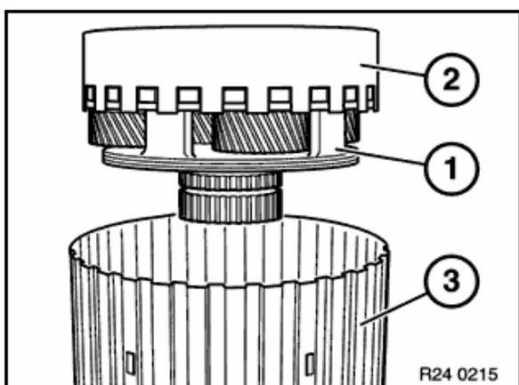
Remove planet spider I (1) and ring gear II (2) from ring gear I (3).
