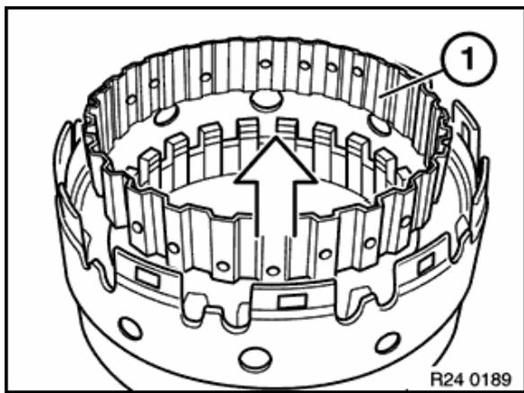
Remove internal disc carrier B (1).
