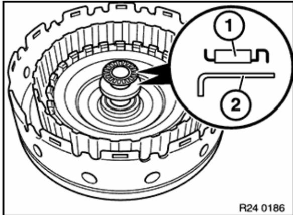
Remove axial needle bearing (1) and angled disc (2) from cylinder C (3).
