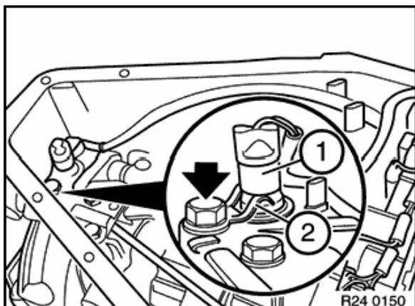
Unfasten screw and remove impulse sensor (1) and retaining clip (2).
