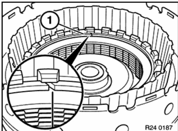
Lift snap ring (1) out of A clutch.
