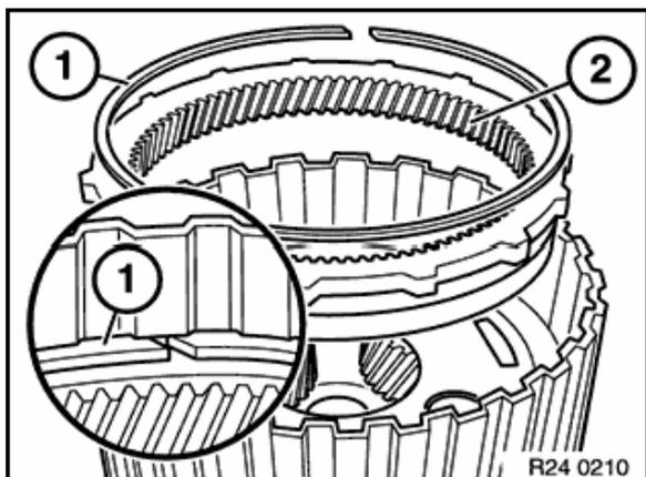
Place planetary gear set I + II on two wooden blocks
