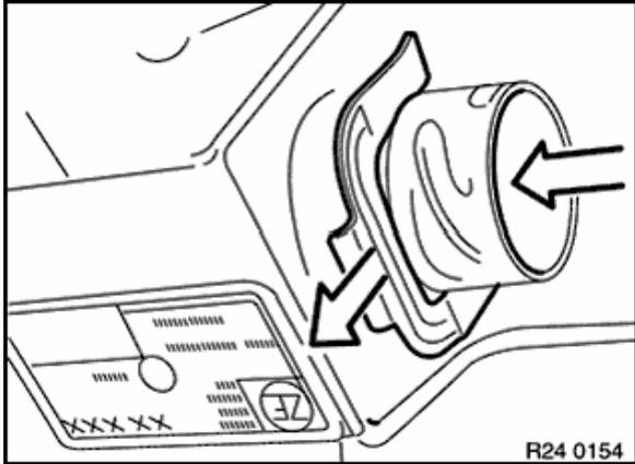
Remove retaining clip and press cable connector into transmission case.
