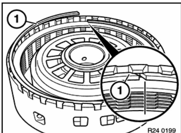
Lift out snap ring (1) from multi-disc brake D and remove complete disc pack.
