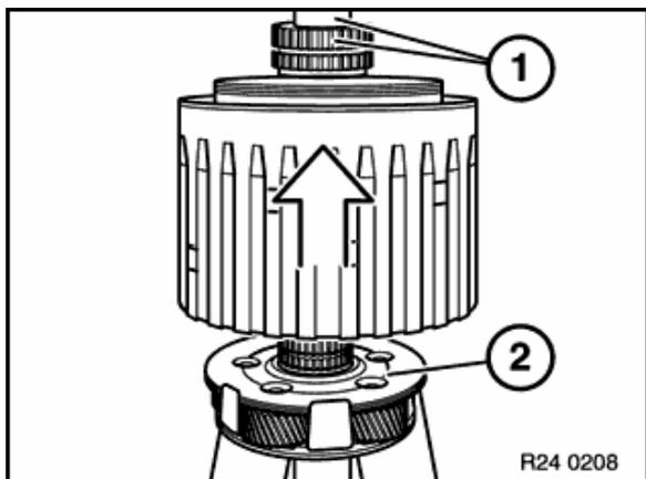
Lift planetary gear set I + II (1) off planetary gear set III (2).
