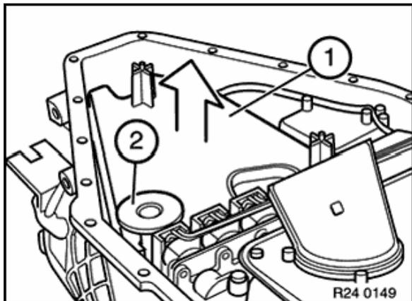
Remove oil container (1) with magnetic disc (2).
