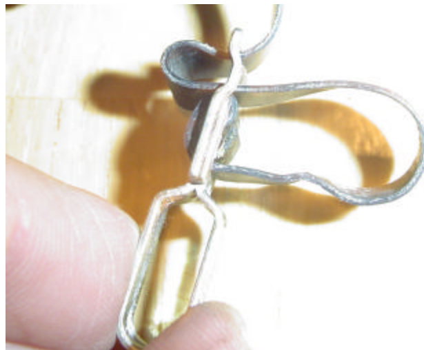
Figure 18 - Detail of control belt threading through clevis
