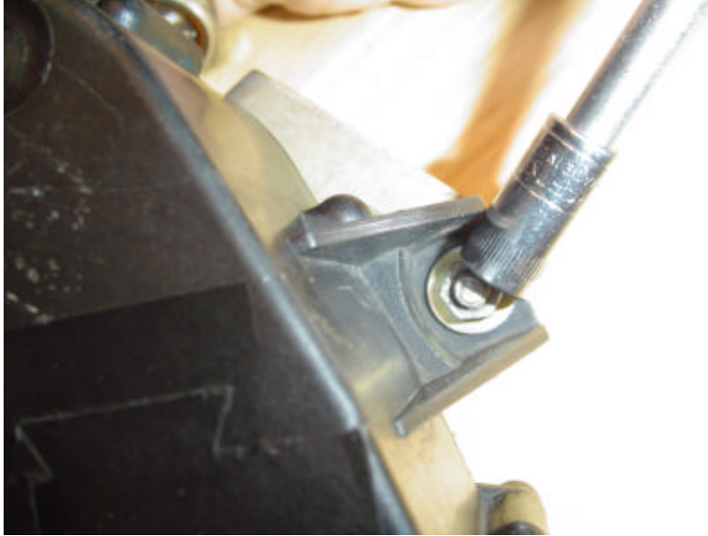
Figure 13 - Remove mounting plate nuts
