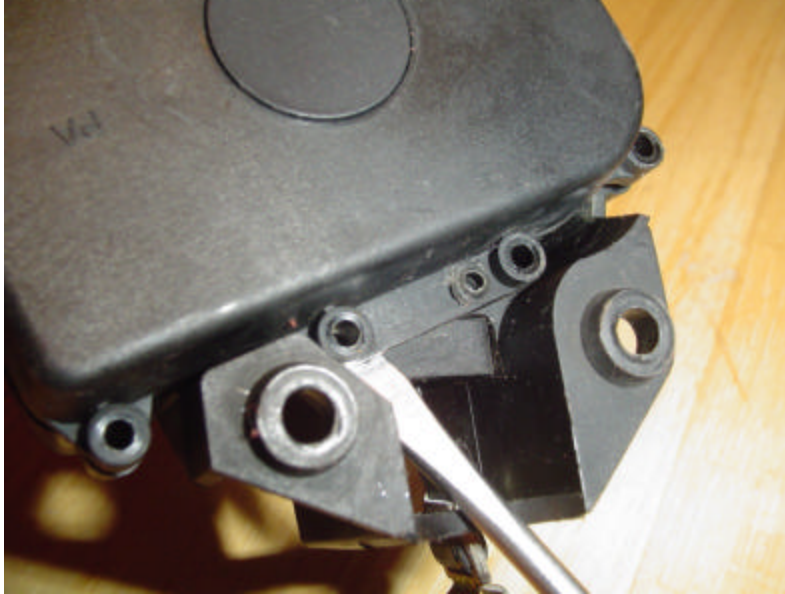
Figure 15 - Using screwdriver to separate shell halves
