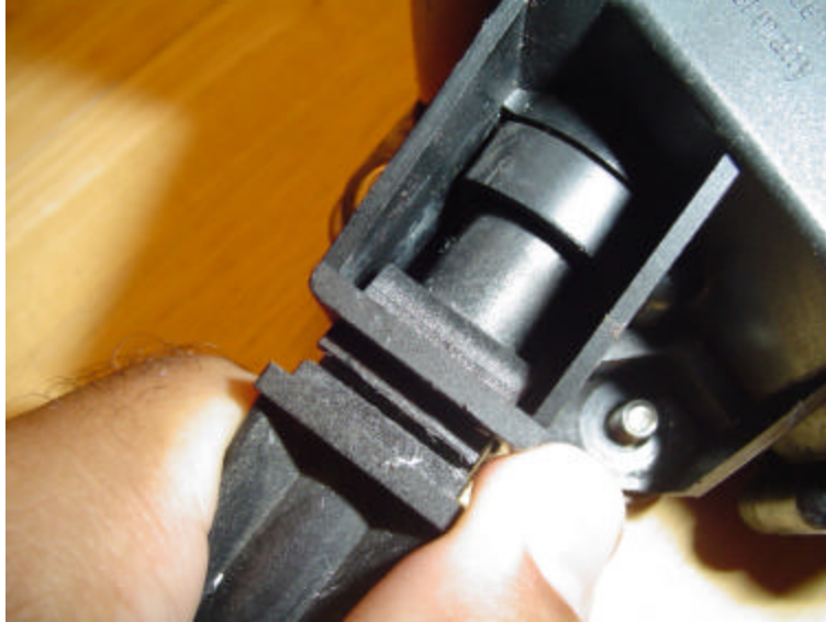
Figure 10 - Sliding out throttle cable
