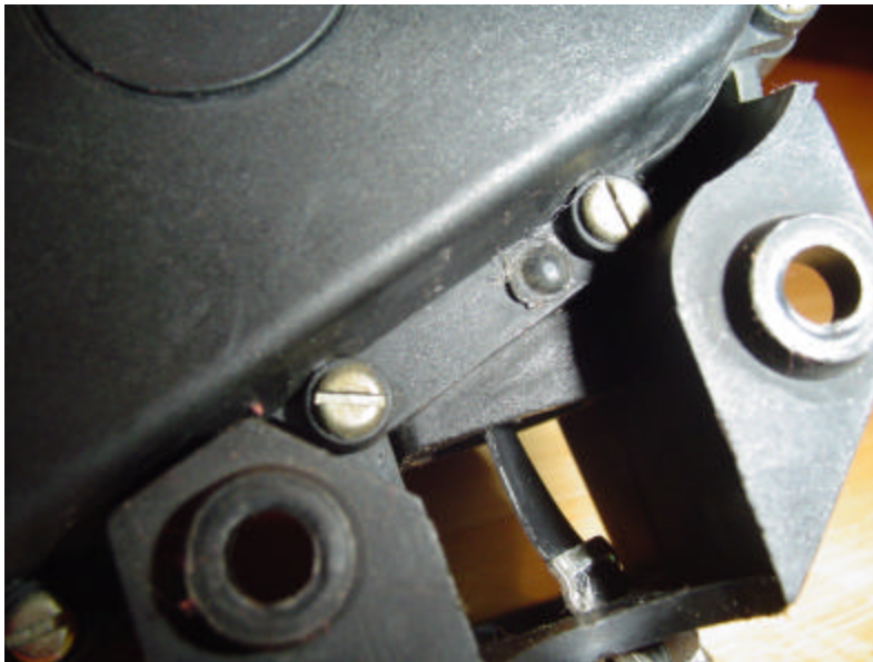
Figure 14 - Remove shell perimeter screws
