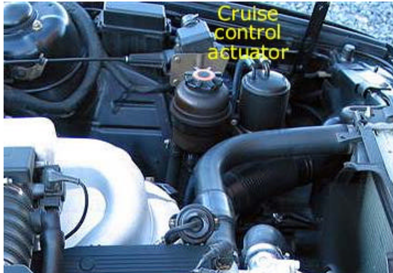
Figure 25 – Typical E34 mounting (non-540i)
