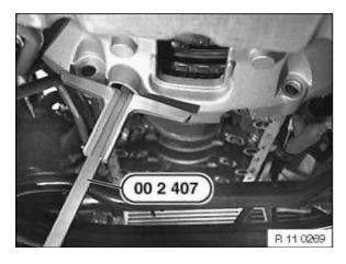
Use special tool 00 2 407 or 00 2 550 to determine depth to flywheel pulse gears.
