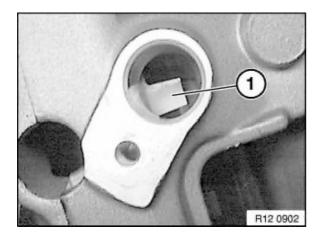
Crank engine at front central bolt so that a full pulse tooth (1) can be seen through opening in removed pulse generator. Make sure that the pulse tooth (1) is exactly centered in the hole.
