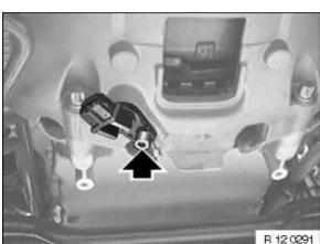
Unscrew screw. Remove impulse sensor.
