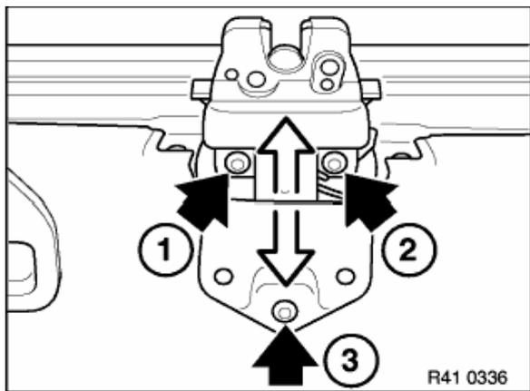
Unfasten retaining screws from upper section of trunk lid lock until only its height can be adjusted.
