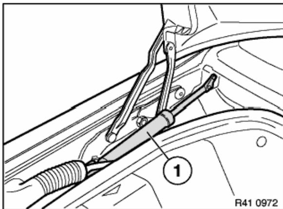
Place hydraulic cylinder (1) in water gutter.
