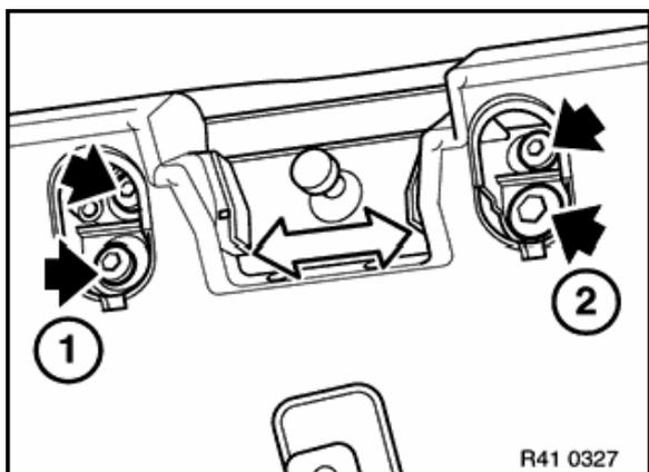
Loosen lower section of trunk lid lock on screws (1) and (2) until
