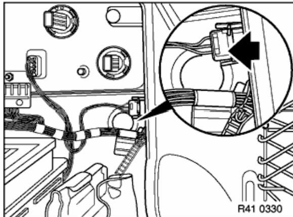
Open right side panel on luggage compartment and disconnect plug connection to actuator motor for the eccentric pin in lower section of trunk lid lock.
