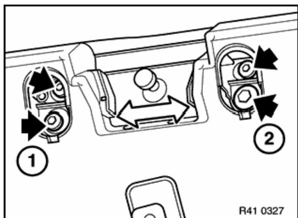
Contact pattern of upper section of trunk lid lock on eccentric pin can be adjusted by inserting or removing washers from retaining screws on lower section of trunk lid lock.
