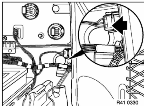
6. Refit plug connection to actuator motor for eccentric pin in lower section of trunk lid lock.
