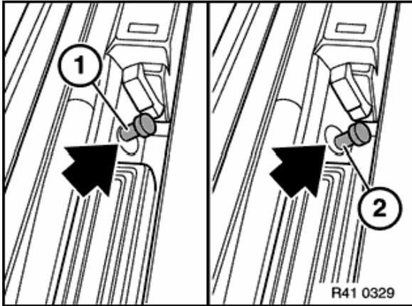
This figure displays the side view of the eccentric pin in the lower section of the trunk lid lock
