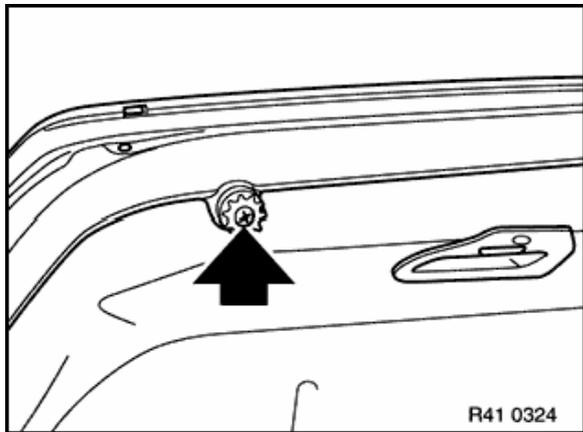
5. Gently twist ejector in detent buffers to right with Phillips screwdriver. This unlocks the detent buffers, enabling ejector to emerge.
