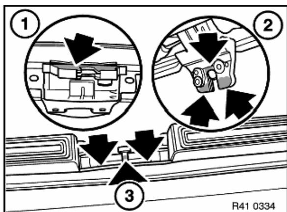
3. Check contact pattern of upper section of trunk lid lock - e.g. coat with grease.
