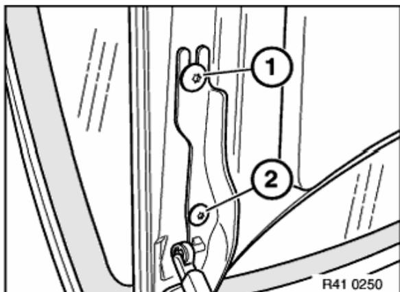
Loosen left and right screws (1) and (2) to point where it is still
