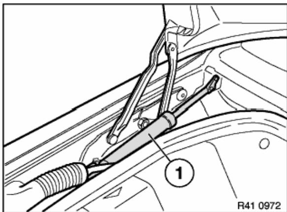
Close trunk lid carefully in order to check that the hydraulic cylinder or the trunk lid is not damaged during closing.
