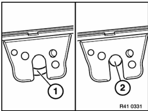
Insert central key in and twist to left: this unlocks upper section of trunk lid lock.
