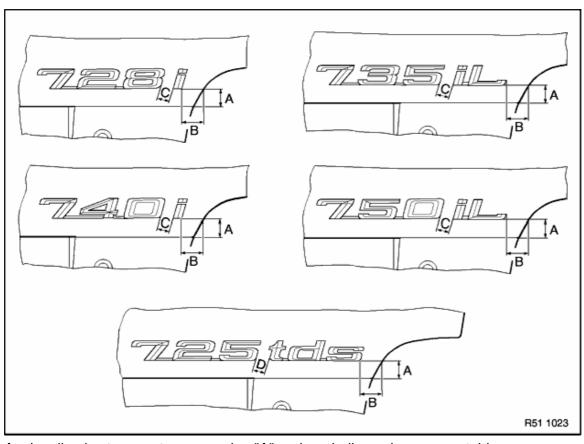
Apply adhesive tape up to upper edge "A" and mark dimensions as per table.
