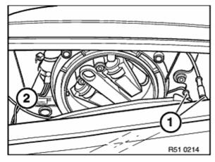
If applicable, remove connector (1) (mirror glass heating). Unlock connector (2) (only 1 detent hook at front) and pull downwards to remove.
