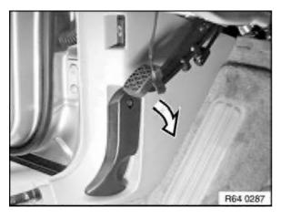
Remove center console, refer to 51 16 200 Remove steering column, refer to 32 31 090 Remove left-hand side trim panel. Remove left support pipe.
