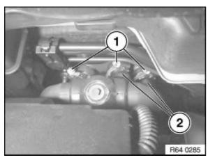
Unfasten hose clips (1) on bulkhead and pull off water hoses. Carefully blow through supply lines (2) to remove the remaining coolant from the heater core.
