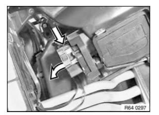
Lever out actuator motor for left footwell flap.
