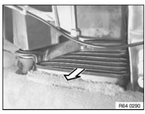
Remove left and right rear air duct.
