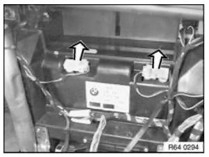
Unclip and remove temperature sensor. Cut open cable ties on the cover.
