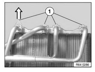
When replacing the heater core, pull out retaining clips (1) and reroute wires.
