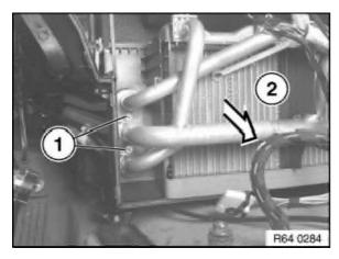
Unfasten screws (1) and pull out heater core (2).
