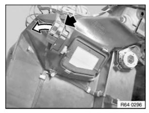
Pry out actuator motor for right footwell flap.
