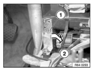
Unfasten screws (1), loosen nut (2) and pry out left and right bracket.
