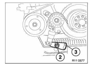
Loosen nuts (2 and 3) and remove compressor drive belt.
