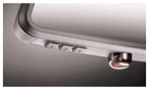
The signal of an original hand held transmitter can be programmed to one of the three channel buttons. The device is operated with the programmed channel button. The integrated universal remote control uses radio frequencies only (not infrared). Transmission of the signal is indicated by the indicator LED.
