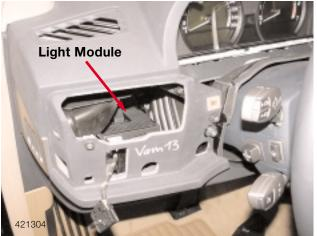
The light module is located below the drivers side of the instrument panel, to the left of the steering column and behind the sheet metal support for the dashboard.
