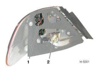
A three-part light assembly is integrated into the luggage compartment lid.
