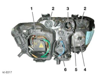
There are holes for easy access to the screws for height adjustment and lateral adjustment of the low-beam and high-beam headlights.
