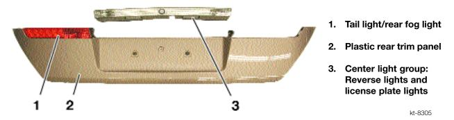
These three lights are secured to the rear lid trim panel on the luggage compartment lid by screws.
