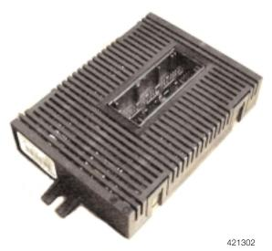
The LM has one 76 pin connector (X12). The case is ventilated to dissipate heat from the final stage semi-conductors.
