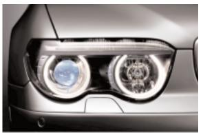
A sidemarker (U.S. version) is integrated into the turn signal indicator.
