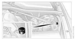
Attach the second end of the cable to the negative terminal of the battery or to the engine or body ground of the vehicle to be started.
