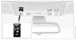
Briefly press the switch: The sunroof opens and the sliding visor moves back approx. 2 in/5 cm or press the switch twice past the resistance point toward the rear: The sunroof opens and the sliding visor moves completely back.
