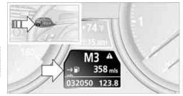
To display the information, press the BC button in the turn signal lever from radio readiness.
