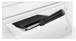
Insert the Allen wrench as far as possible into the opening and turn firmly in the direction indicated by the arrow until the rear window is completely open.
