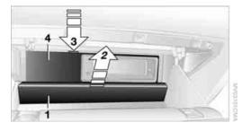
Press the coupling downward, arrow 3, and fold the lid 4 forward.
