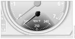
During normal operation, the engine oil temperature is between approx, 160 °F /70 °C and approx. 340 °F/170 °C.
