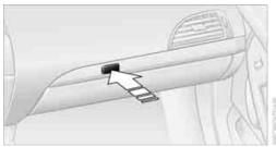
Press the button. The glove compartment opens automatically and the lamps come on.
