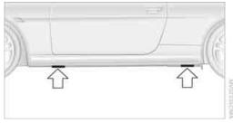
The jacking points for the car jack are located in the positions shown.
