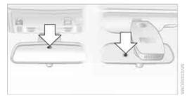
The interior mirror is provided with two photocells to control its automatic dimming function. One is integrated into the mirror glass, refer to arrow, while the other is located at a position slightly offset from this on the back of the mirror housing.
