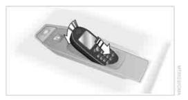
The mobile phone's battery is charged with the ignition lock at radio readiness or higher or with the steering unlocked.
