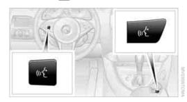
In This symbol on the Control Display and an acoustic signal tell you that the voice command system can respond to commands.
