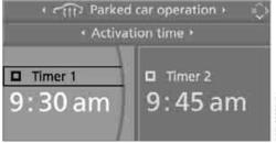
6. Select the time and press the controller. The first time setting is highlighted.
