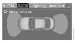
Select "PDC display on" and press the controller.
