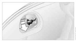
Bulb 21 watts, PY 21 W
