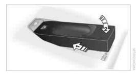
To remove the snap-in adapter: Press the area 1 around the button.
