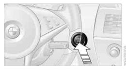
Do not press either the brake or the clutch pedal as long as you do not want to start the engine. The engine starts immediately when you briefly press the Start/Stop button and press the brake pedal with an automatic transmission, or the clutch pedal with a manual transmission.
