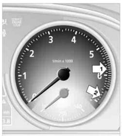
The white-striped advance warning field, arrow 1, changes depending on the engine temperature. The segments disappear in sequence as the engine warms to its normal operating temperature.
