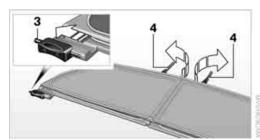
4. Unfold the rear mounts 4.
