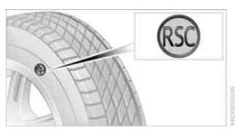
You will recognize run-flat tires by the circular symbol containing the letters RSC on the side of the tire.
