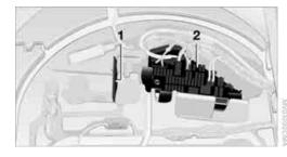
Fold the cover under the floor mat upward and remove the bracket for the onboard tool kit. Information on fuse allocation 1 and additional fuses 2 are provided there.
