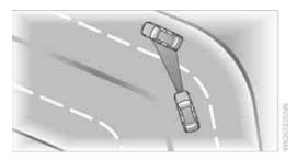
In approaching a curve, it is possible that active cruise control would react briefly to a vehicle in the adjacent lane. In addition, the system can sense if your vehicle is in a curve and may not accelerate. If your vehicle decelerates in either case, you can choose to overcome the deceleration by briefly pressing the accelerator pedal.
