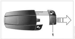
Press the button 1 to unlock the key.
