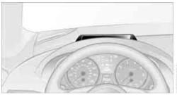
Only clean the cover of the Head-Up Display with a soft, lint-free cloth or with a display cleaning cloth, otherwise damage may result.◀
