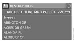
Turn the controller to the right until the request for the entry of a street in the country appears and press the controller.
