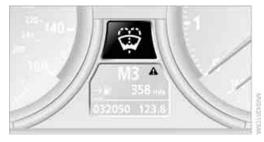
▲ This symbol means that a Check Control message has been generated. The symbol remains visible even if the Check Control mes-
