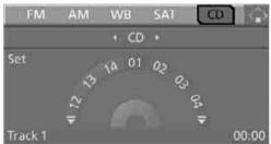
On vehicles with a CD changer, change to the second field from the top and turn the controller until "CD" is selected and press the controller.
