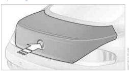
Press the upper half of the BMW emblem or press the button on the remote control for approx. 1 second: the luggage compartment lid opens.
