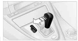
Move the selector-lever from position D to the left into shifting slot M/S:
