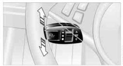
Press the lever up or down. The displays in the instrument cluster disappear.
