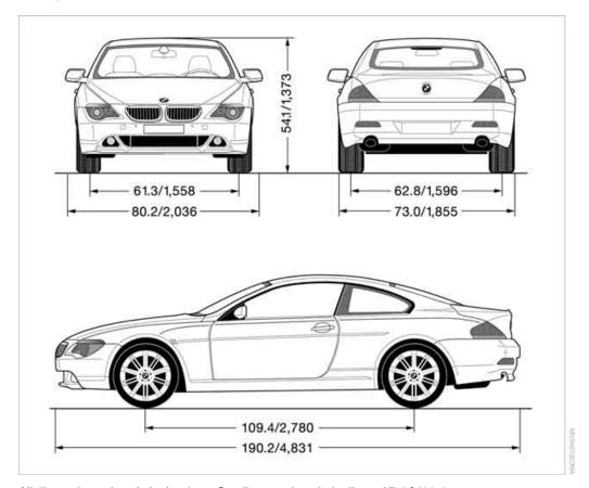
All dimensions given in inches/mm. Smallest turning circle diam.: 37.4 ft/11.4 m
