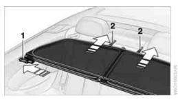
Guide the rear mounts 2 into the receptacles provided. Push the securing pin 3 on the left side into the appropriate opening until it snaps into place.
