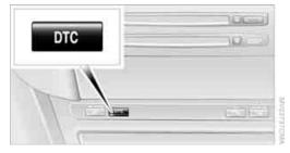
Press the button until the DSC indicator lamp in the instrument cluster lights up, but not for longer than approx. 10 seconds. DTC Dynamic Traction Control and DSC are deactivated together. Interventions promoting stability and forward momentum will no longer be carried out. The stability-promoting intervention of the active steering\* is also deactivated, refer to page 92.
