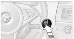
Briefly pressing the Start/Stop button several times switches the radio readiness or the ignition on and off.
