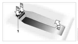
2. Insert the snap-in adapter at the front and press down until it engages.
