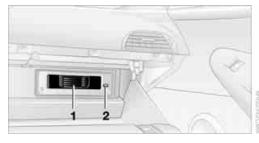
Press button **2** to eject the CD magazine **1**. Wait at least 2 seconds before pushing in the
