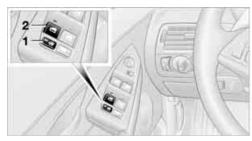
1. Briefly press button 1: The LEDs in the button 1 and the switch 2 light up for approx. 10 seconds.
