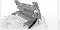
Do not carry out the next operation, raising top ends, until the top has been swung forward, as otherwise damage can occur.◀
