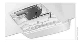
Use the Allen wrench to move the glass sunroof in the desired direction.
