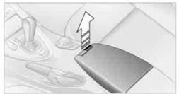
Pull the right button: Move the armrest upward or downward and lock it in the desired position.
