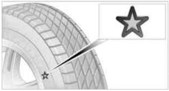
BMW recommends particular tire brands for each tire size. You can recognize these from the clearly visible BMW marking on the tire sidewall.
