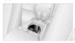
The compartment of the rear center console contains a built-in cup holder and a removable one.
