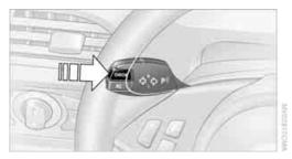
To hide these Check Control messages: Press the CHECK button on the turn signal lever.
