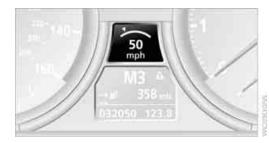
The speed currently being driven is stored and maintained. It is indicated on the speedometer and briefly in the instrument cluster.
