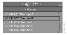
The channel is stored. The stations of the last selection criterion are displayed again after a short time.
