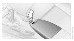
A storage compartment is located in the armrest between the front seats. This compartment is integrated into the central locking system and can also be locked separately using the hotel function, refer to page 33.
