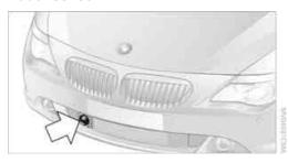
Heavy rain, dirt, snow, or ice can impair the detection of vehicles ahead. If necessary, clean the radar sensor under the front bumper. In doing so, be especially careful when removing layers of snow and ice.
