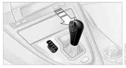
An interlock prevents inadvertent gearshifts into selector-lever positions R and P. To cancel the interlock, press the button on the front of the selector-lever knob, refer to arrow.
