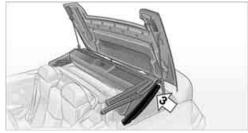
Together with the other person, pull the two sides of the convertible top out simultaneously and pivot forward. When doing so, keep the convertible top compartment lid open, arrow 4, e.g. with your shoulder.
