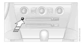
Press the button if the sound output is switched off.
