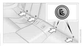
The mountings for the LATCH child-restraint fixing system are located under the points marked with the symbols. They are not visible from the outside.
