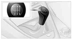
When shifting into 5th/6th gear, press the selector-lever toward the right, otherwise an inadvertent shift into 3rd or 4th gear could lead to engine damage. ◀
