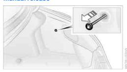
In the event of an electrical malfunction, you can release the fuel filler door manually:
