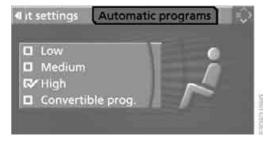
Select the desired intensity and press the controller.
