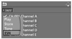
Select "ESN" and press the controller. The electronic serial number, ESN, is displayed.
