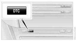
Press the button; the DTC indicator lamp in the instrument cluster lights up.
