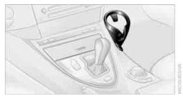
The removable cup holder can be inserted into the side of the center console.
