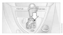
Using the screwdriver from the onboard toolkit, refer to page 201, press the lever at the point marked in red and move the selector lever into the desired position.
