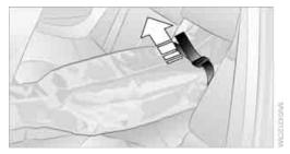
After loading, secure the ski bag and its contents. To do so, tighten the retaining belt at the buckle.
