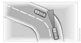
Because of the limited range of the system, it is possible that in curves or on the peaks and valleys of hilly roads, a vehicle ahead may be recognized late, or not at all. Therefore, it is up to the driver to select a speed that is prudent in view of the curves and terrain of the roadway.
