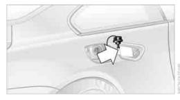
Place the fuel filler cap in the bracket attached to the fuel filler door.
