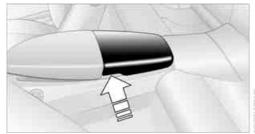
To open, raise the cover at the left or right edge. The compartment contains the cup holder and the lock for the hotel function, refer to page 33.
