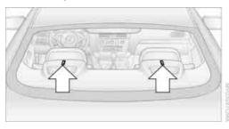
There are two additional mounting points for child restraint systems with a tether strap, refer to arrows.
