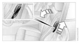
Pull the lever upward and fold the backrest forward.
