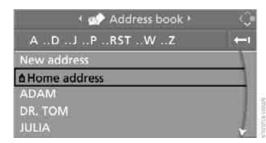
Select "Use current location as address", or "Save current destination" during the destination guidance, and press the controller. To select the home address as the destination:
