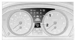
Indicator and warning lamps can light up both in the display area **1** and in the display **2** in various combinations and colors.
