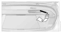
With the convertible top closed, you can enlarge the luggage compartment capacity. To do so, unfold the handle and press it downward in the direction of travel, refer to arrow. This moves the convertible top compartment floor into the raised position.
