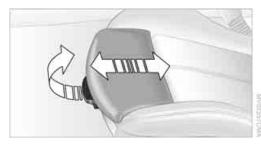
Pull the lever and adjust the thigh support in the longitudinal direction.
