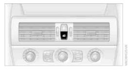
This button serves to unlock or lock doors and the luggage compartment lid, but does not activate the anti-theft system. The fuel filler door remains unlocked.
