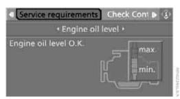
5. Change to the second field from the top if necessary. Turn the controller until "Engine oil level" is selected and press the controller. The oil level is displayed.
