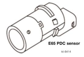
The design of the sensor varies from that used until now in that the outer membranes are completely round instead of oval.
