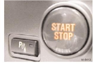
The button can be used to activate or deactivate PDC manually. The locating light is connected to terminal 58g. The function indicator LED is connected to the control unit.
