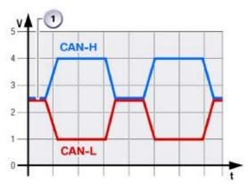
These values are approximate values and can vary by a few hundred milli-volts [mV] depending on the bus load. Oscilloscope settings for the measurement of the PT-CAN (or any fast CAN, i.e. 500 Kbps):
