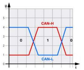
These values are approximate values and can vary by a few hundred milli-volts [mV] depending on the bus load. Oscilloscope settings for the measurement of the K-CAN:
