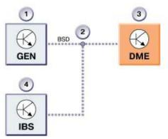
Bit-serial data interface example.
