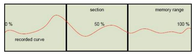
As long as the reference and differential cursors are displayed (with channel CH1 or CH2 in the "Cursor" settings group selected), the section can only be displaced between the two cursors. To scroll through the entire memory, you have to deselect both channels in the "Cursor" settings group
