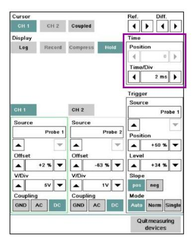
By increasing the sampling rate with the "<Time>/Div" arrow keys, you can zoom in further into a curve section until the curve is completely expanded.
