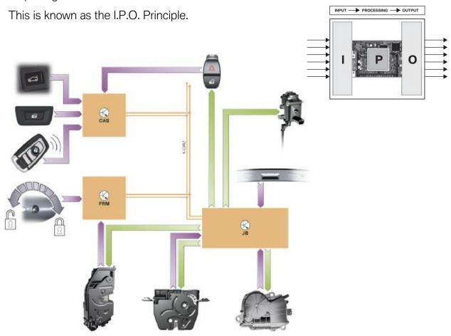
Any device controlled by a processor requires input to the alert the operating program of a condition. The program processes the input information and logically activates an output of a component.
