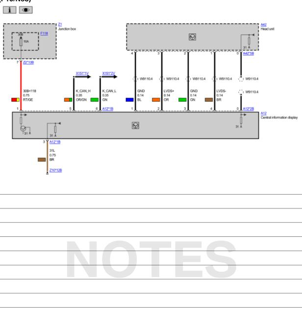
All other wiring have a color label in a rectangle next to the wiring color. The distribution of color labels in the rectangular represent the actual color of the wiring. The wiring diagrams for further series will be displayed in color as well.
