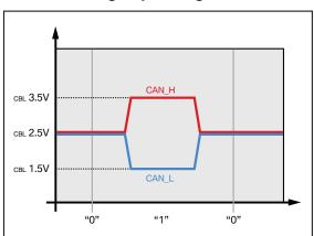
The figures shows the two levels of data transmission in both the High-speed and Low-speed CAN's.
