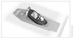
The mobile phone's battery is charged from radio readiness or with the steering unlocked.
