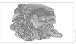
With a 305 cu in/5 liter displacement, the highspeed V10 engine generates a maximum output of 373 kW and a maximum torque of 384 lb ft/520 Nm. Its spontaneous response characteristics yield a very broad usable engine speed range. At the maximum engine speed of 8,250 rpm, the flow of fuel is interrupted in order to protect the engine. Due to the powerful engine dynamics, when the vehicle is at rest, the maximum engine speed is limited to 7,000 rpm.
