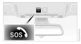
Press the SOS button for at least 2 seconds. The LED in the button lights up. As soon as the voice connection to the BMW Assist Response Center has been established, the LED flashes.
