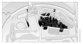
Fold the cover under the floor mat upward and remove the bracket for the onboard tool kit. Information on fuse allocation **1** and additional fuses **2** are provided there.
