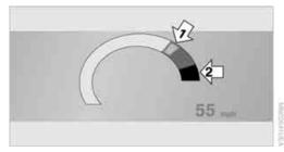
To achieve the best vehicle acceleration with a sporty driving style, shift lights in the Head-Up Display\* indicate the optimum shifting point briefly before reaching the maximum rpm. Refer to Shift lights, page 65.
