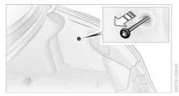
In the event of an electrical malfunction, you can release the fuel filler door manually:
