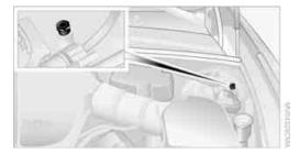
5. Attach the second end of the cable to the negative terminal of the battery or to the engine or body ground of the vehicle to be started.
