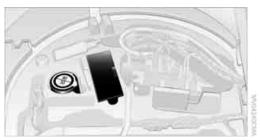
The M Mobility System is located in the cargo bay under the floor panel flap.
