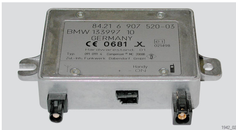
Fig. 40: Aerial line compensator for ULF
