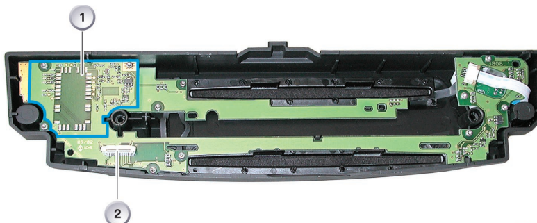
Fig. 20: Rear view of front panel with Bluetooth module
