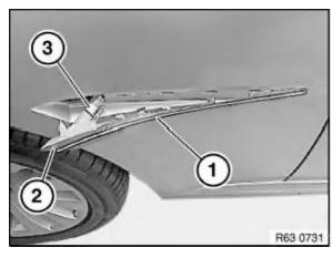
Remove trim strip (1) from front auxiliary turn signal lamp (2). Unfasten plug connection (3) and disconnect. Remove front auxiliary turn signal lamp (2).
