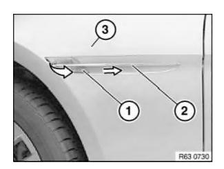
Slide front auxiliary turn signal lamp (1) with trim strip (2) towards rear and fold out in direction of arrow from front side panel (3).
