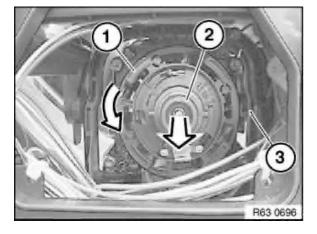
Turn retaining ring (1) in counterclockwise direction and remove.
