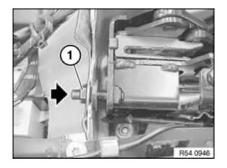
Fixing convertible top adjustment made:
