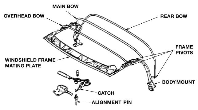
Regardless of the mode of automation, the mechanical pivot points and movement while raising or lowering are the same for both variations.
