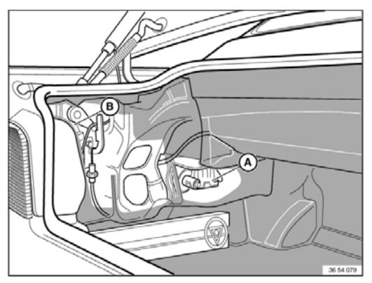
• **FULL AUTO ONLY:** Top Lock Motor with flexible drive tubes and lock drive mechanisms. The lock drive mechanisms also activate the off tension linkage rods for automatically moving the top to the off tension position.
