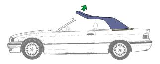
After the windows have been lowered slightly, the top is released from windshield frame.
