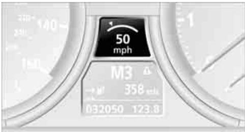
The speed currently being driven is stored and maintained. It is indicated on the speedometer and briefly in the instrument cluster.
