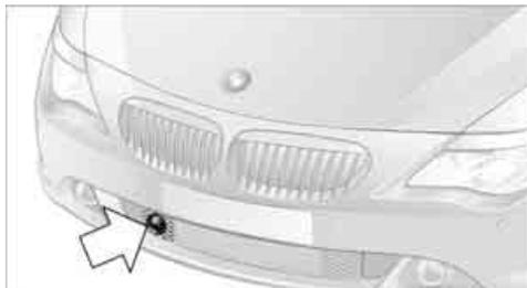
Heavy rain, dirt, snow, or ice can impair the detection of vehicles ahead. If necessary, clean the radar sensor under the front bumper. In doing so, be especially careful when removing layers of snow and ice.
