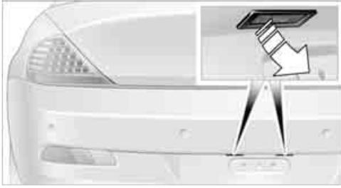
Bulb 5 watts, WY 5 W
