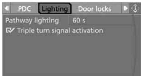
5. Select "Triple turn signal activation" and press the controller.
