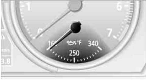
During normal operation, the engine oil temperature is between approx. 160 °F/70 °C and approx. 340 °F/170 °C.
