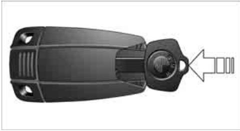
Remove the adapter from the holder in the glove compartment and slide the spare key into the adapter before use.
