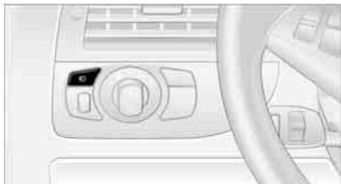
The parking lamps or low beams must be switched on for the fog lamps to operate. The green indicator lamp in the instrument cluster lights up when the fog lamps are switched on. The fog lamps are switched off whenever the high beams are switched on.
