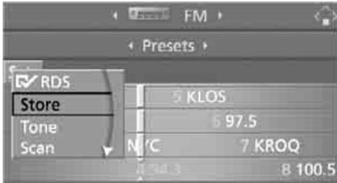
5. Turn the controller until the desired memory position is selected.
