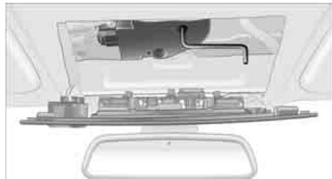
3. Use the Allen wrench to move the sliding visor in the desired direction.
