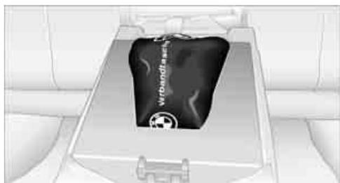
**!** To refit the filler element, insert the two bottom tabs into the strip and press the filler element back into place. Make sure that you do not damage the rear seat upholstery. ◀
