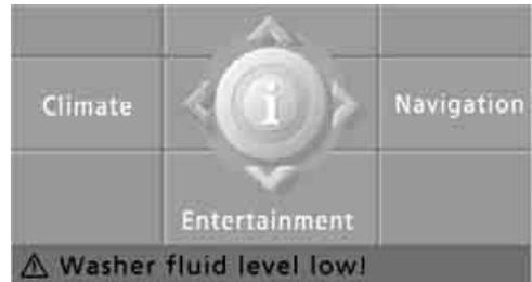
Text messages at the bottom edge of the Control Display explain the meaning of the indicator and warning lamps displayed.
