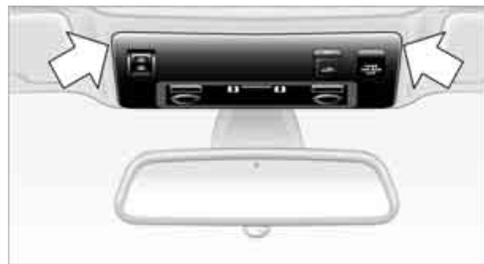
2. Insert the Allen wrench supplied with the onboard tool kit into the opening provided.
