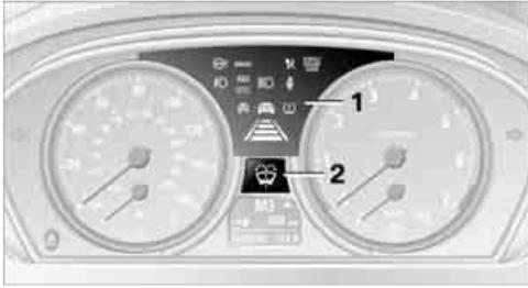
Indicator and warning lamps can light up both in the display area **1** and in the display **2** in various combinations and colors.
