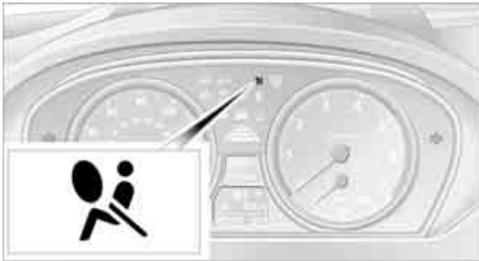
From radio readiness, refer to page 58, the warning lamp lights up briefly, indicating the operational readiness of the entire airbag system and the safety belt tensioners.
