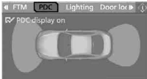
5. Select "PDC display on" and press the controller.
