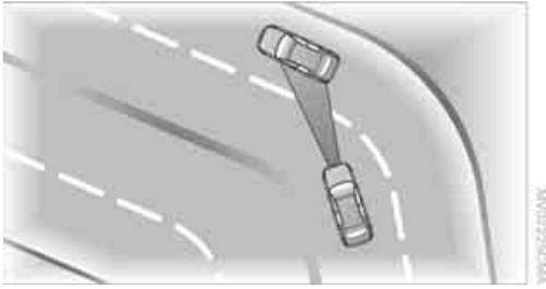
In approaching a curve, it is possible that active cruise control would react briefly to a vehicle in the adjacent lane. In addition, the system can sense if your vehicle is in a curve and may not accelerate. If your vehicle decelerates in either case, you can choose to overcome the deceleration by briefly pressing the accelerator pedal.
