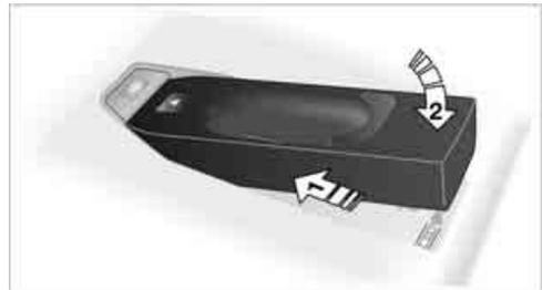
To remove the snap-in adapter:
