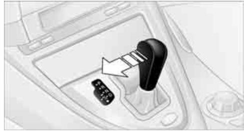
Move the selector-lever from position D to the left into shifting slot M/S:
