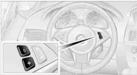
You can program the buttons individually. The setting is stored for the remote control currently in use. iDrive, for explanation of principle, refer to page 16.
