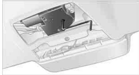
3. Use the Allen wrench to move the glass sunroof in the desired direction.
