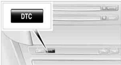
Press the button until the DSC indicator lamp in the instrument cluster lights up, but not for longer than approx. 10 seconds. DTC Dynamic Traction Control and DSC are deactivated together. Interventions promoting stability and forward momentum will no longer be carried out. The stability-promoting intervention of the active steering\* is also deactivated, refer to page 92.
