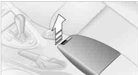
A storage compartment is located in the armrest between the front seats. This compartment is integrated into the central locking system and can also be locked separately using the hotel function, refer to page 33.
