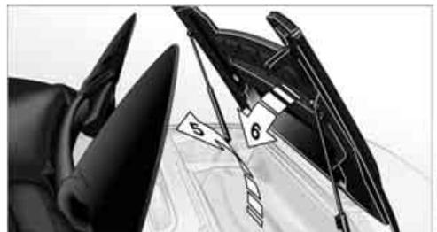
5. Fold the top ends down onto the convertible top compartment lid.
