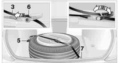
5. Completely open the tensioning lock.
