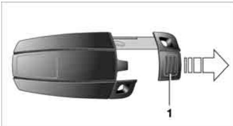
Press button 1 to unlock the key.
