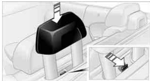
2. Press the rollover protection unit halfway down from above.
