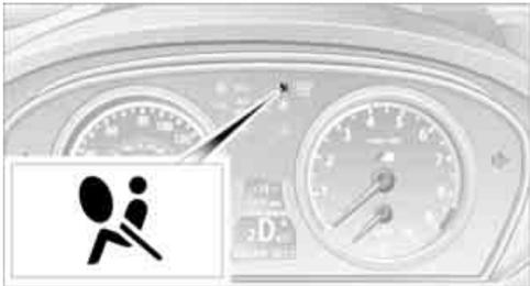
From radio readiness, refer to page 60, the warning lamp lights up briefly, indicating the operational readiness of the entire airbag system and the safety belt tensioners.
