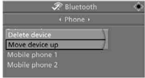
The selected mobile phone is moved upward by one position.
