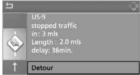
Select "Detour" and press the controller. The navigation system determines a new route to avoid the traffic jam.
