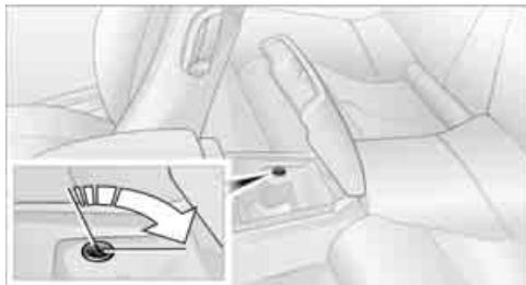
Turn the key to the right, refer to illustration, until the key slot points in the direction of travel and then remove:
