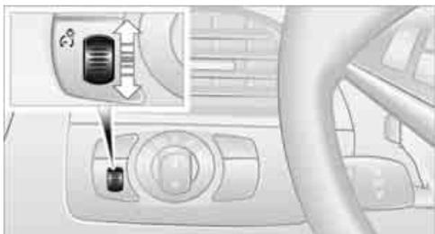
The lighting intensity can be adjusted with the knurled wheel with the parking lamps/low beams switched on.
