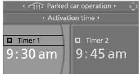
6. Select the time and press the controller. The first setting of the time display is selected.
