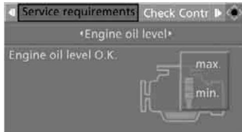
6. Change to the second field from the top if necessary. Turn the controller until "Engine oil level" is selected and press the controller. The oil level is displayed.
