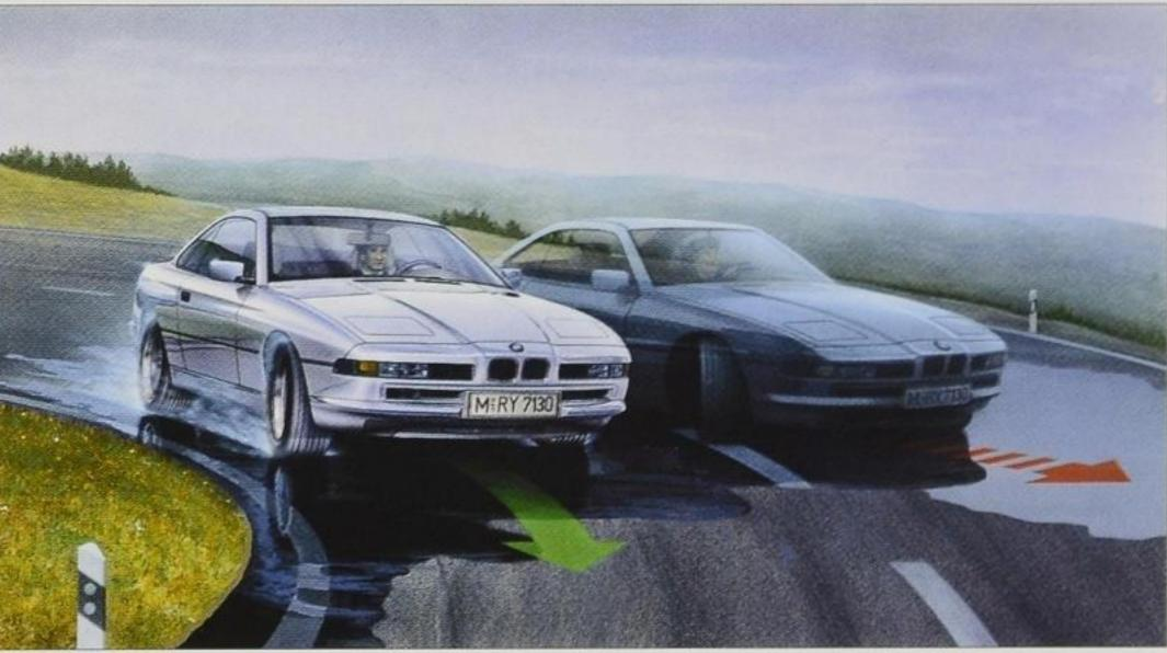
A standard feature of the 850CSi, the dynamic driving system with active rear axle kinematics provides a quantum leap in driving stability and maximum safety even in extreme situations.
