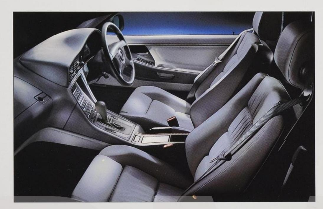
BMW sports seats for the driver and front passenger assure optimum side support even at high speeds on winding roads. Even the thigh support and seat angle on the front passenger's side can be adjusted, all adjustment functions naturally being electric. As a further feature, the driver's seat is also available with memory function. BMW sports seats are not available in conjunction with the lumbar support.
