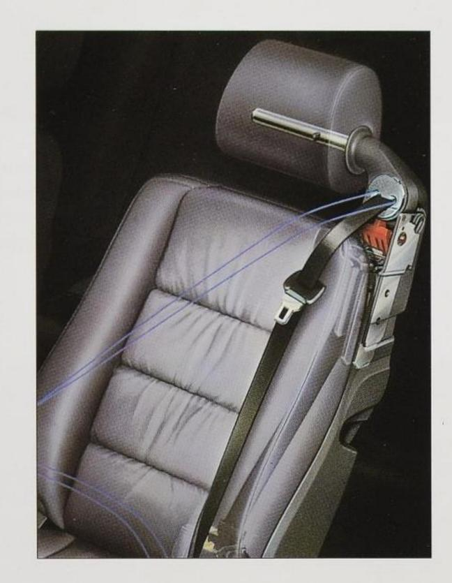
With the seat-integrated belt system all three belt pivot points move together with the seat when adjusted. As a result, you always have optimum restraint and protection regardless of your size and seating position.
