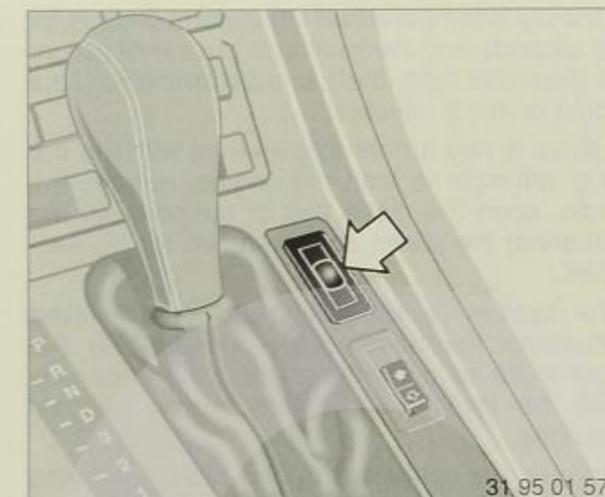
**Anti-theft alarm system with additional interior protection and tilt alarm sensor\***
