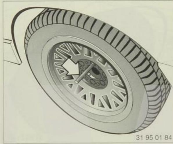
9. Screw in the remaining wheel studs and tighten them all in a crosswise pattern.
