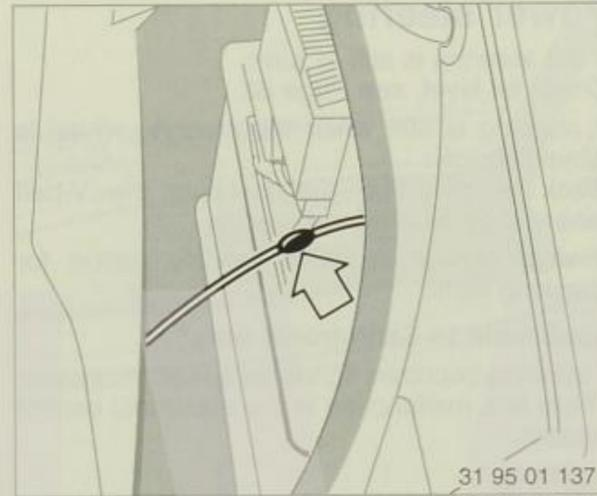
Before detaching the right luggage compartment trim, first disconnect the plug connection for manual fuel filler flap release at the pull wire (arrow).
