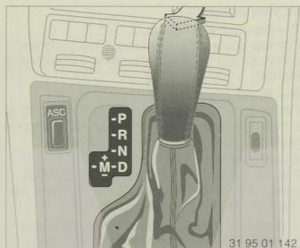
There is a locking catch on the front of the selector lever handle, which prevents the lever from being moved accidentally to positions R and P. Press this catch to release.
