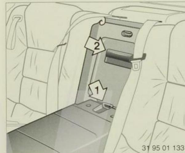
Press the release catch (arrow 1): this will release the loading flap in the luggage compartment.
