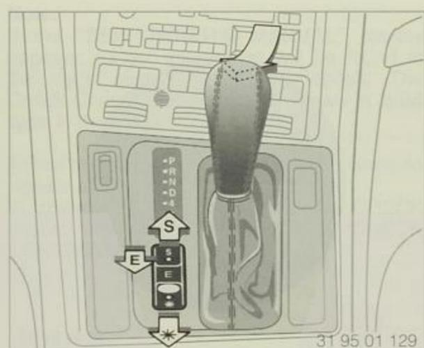
There is a locking catch on the front of the selector lever handle, which prevents the lever from being moved accidentally to various positions. Press this catch to release.
